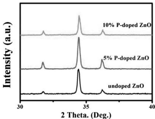
**Figure 2.** XRD pattern of 5% P-doped ZnO, 10% P-doped ZnO nanoparticles and undoped ZnO.
