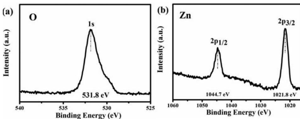
**Figure S1.** XPS spectrum of P-doped ZnO nanoparticles, (a) O spectrum, (b) Zn spectrum.
