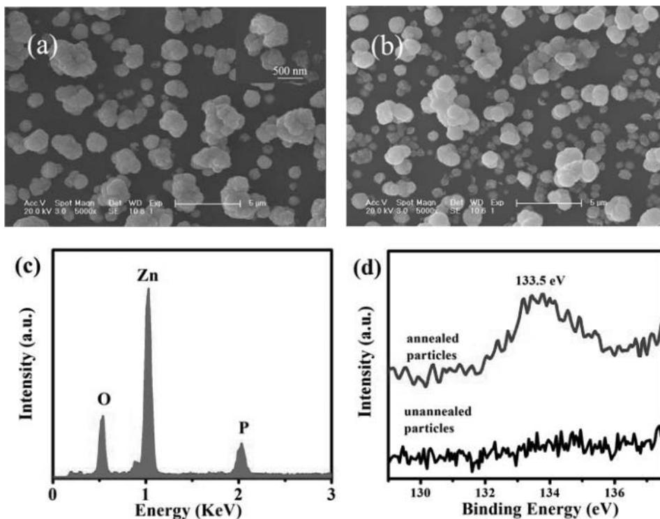
**Figure 1.** (a), (b) SEM images of 5% P-doped ZnO and 10% P-doped ZnO nanoparticles, respectively; (c) EDX spectrum of annealed P-doped ZnO; (d) XPS spectrum of annealed P-doped ZnO and unannealed samples.
