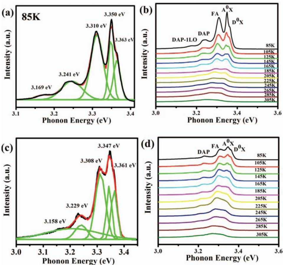
**Figure 3.** (a) Low-temperature PL spectra of 5% P-doped ZnO, (b) temperature-dependent PL spectra of 5% P-doped ZnO, (c) Low-temperature PL spectra of 10% P-doped ZnO, (d) temperature-dependent PL spectra of 10% P-doped ZnO.
