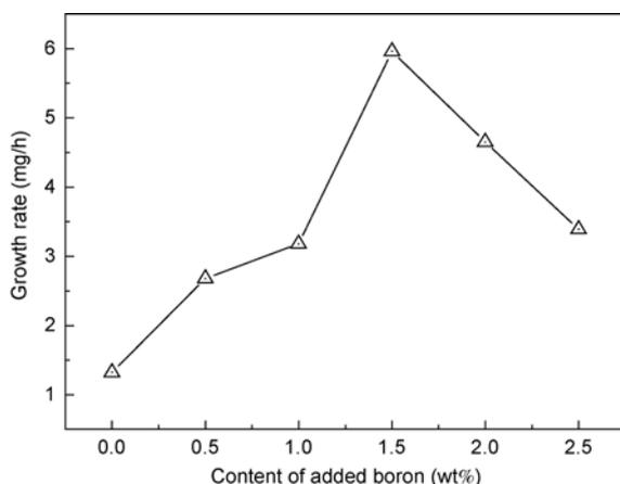
**Figure 4** Curve of growth rate versus the content of added boron.
