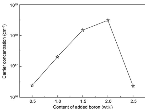
**Figure 6** Carrier concentration vs. content of boron added into the graphite powder.
