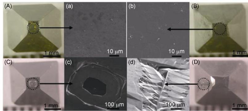
**Figure 2** Optical photos and SEM images of the diamond crystals grown with different added amounts of boron. (A) 0.5 wt%; (B) 1.5 wt%; (C) 2.0 wt%; (D) 2.5 wt%. (a)–(d) are the SEM images of samples (A)–(D).
