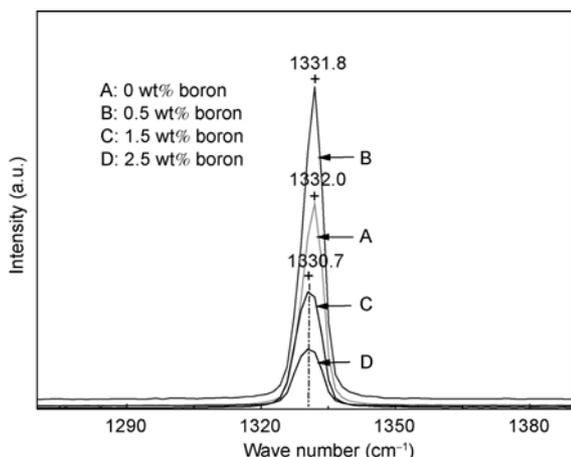
**Figure 5** Raman spectra of the diamond crystals grown with different added amounts of boron.
