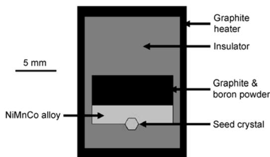
**Figure 1** Sample assembly for diamond growth using temperature gradient method.
