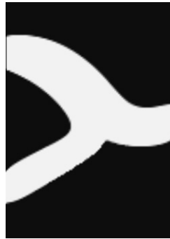
Fig. 13. Optimal design of the three-terminal device for steady flow.
