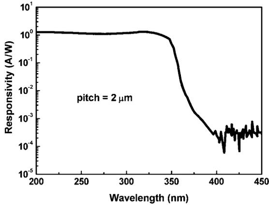
Figure 4. Spectral response of the  $\text{Mg}_{0.4}\text{Zn}_{0.6}\text{O}$  UV detector.
