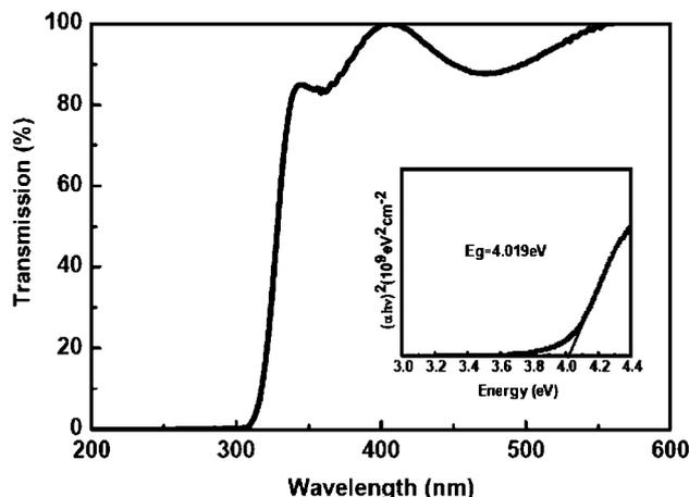
**Figure 2.** Transmission spectra of the  $\text{Mg}_{0.4}\text{Zn}_{0.6}\text{O}$  film. The inset shows  $(\alpha hv)^2$  versus  $hv$  that gives the room temperature band gap.
