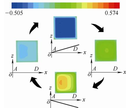
Fig. 7. Tangential velocity cycle variation diagram of the orifice of the spiral tube when the rotation angular velocity  $\Omega = 4 \text{ (m/s)}$
