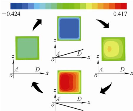
Fig. 5. Tangential velocity cycle variation diagram of the orifice of the spiral tube when the rotation angular velocity  $\Omega = 0 \text{ (m/s)}$
