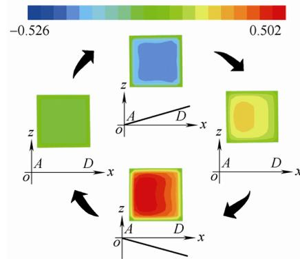
Fig. 6. Tangential velocity cycle variation diagram of the orifice of the spiral tube when the rotation angular velocity  $\Omega = 3 \text{ (m/s)}$
