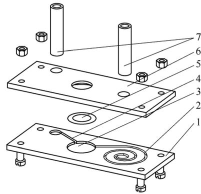
Fig. 3. Structure diagram of the spiral-tube-type valveless piezoelectric pump
