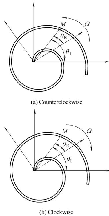
Fig. 1. Diagram of flow in the spiral tube in the rotating reference system
