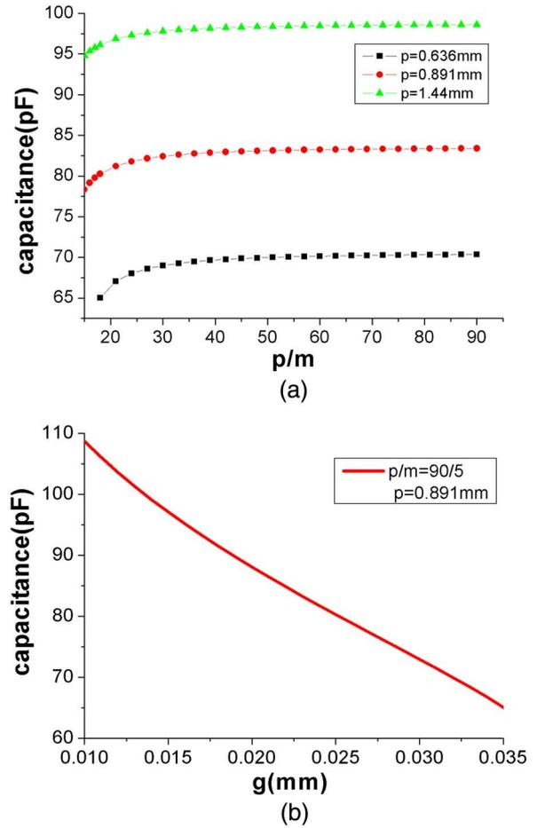
Fig. 6. Calculated inter-electrode capacitance between electrodes  $A_1$  and  $A_2$  (a) with different pitch width and (b) with different insulation gap.
