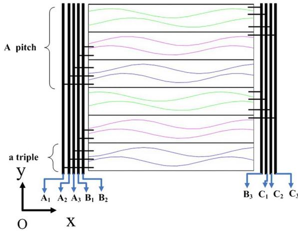
Fig. 1. Schematic of the Vernier anode with two pitches.
