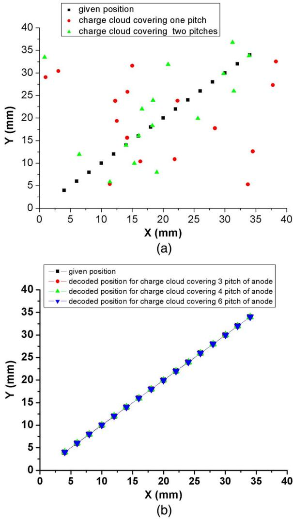
**Fig. 2.** Calculated decoding position when charge cloud covers (a) one to two pitches and (b) no fewer than three pitches for a group of given positions.
