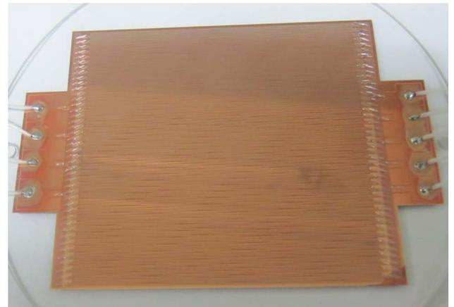
Fig. 7. Photograph of a 38 mm × 38 mm Vernier anode made in copper film on a quartz substrate.
