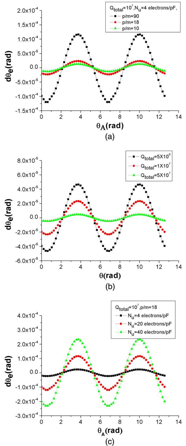
**Fig. 8.** Deviation of triple phase (a) for different  $p/m$ , (b) for different MCP gain, and (c) for different ENC slope.
