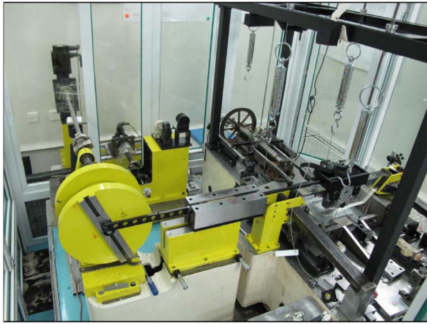
Fig. 6. CIOMP-2 grating ruling engine located in China.
