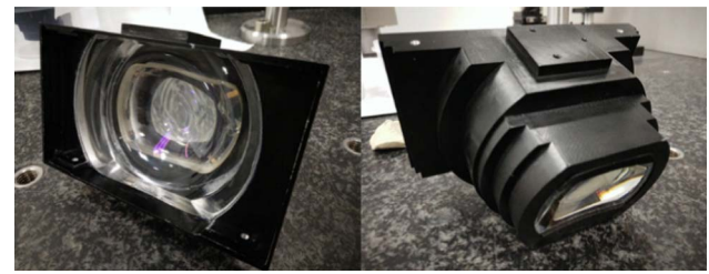
Fig. 7. Image of the HMD monocular optical system.
