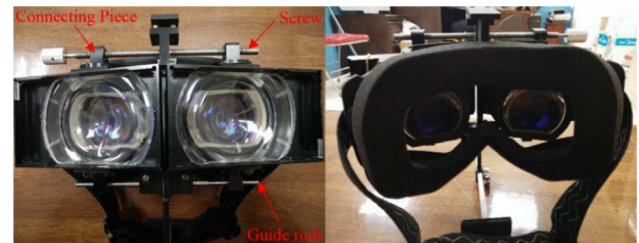
Fig. 8. Assembled HMD binocular optical system.
