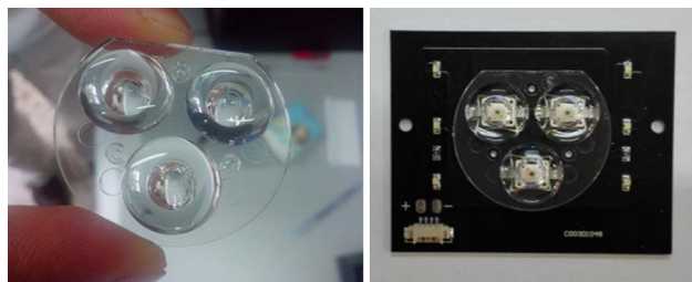
Fig. 12. Completed palm/fingerprint lighting system with near-infrared LED and secondary lens array.
