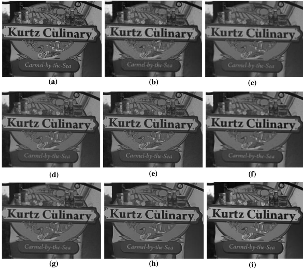
Figure 4. Simulated reconstructed results. (a) HR image (b) LR image (c) NLM method, PSNR = 22.8464, SSIM = 0.7492, Operation time = 53.6721 s. (d) SCSR method, PSNR = 26.3778, SSIM = 0.8649, Operation time = 103.3653 s. (e) BP-JDL method, PSNR = 26.8799, SSIM = 0.8779, Operation time = 197.0814 s. (f) AGMS method, PSNR = 25.3527, SSIM = 0.8219, Operation time = 2.3411 s. (g) Multiple SR method, PSNR = 25.5773, SSIM = 0.8444, Operation time = more than one hour. (h) The proposed method without regularization (Section 3.4). (i) The proposed method, PSNR = 27.3424, SSIM = 0.8988, Operation time = 23.9132 s.
