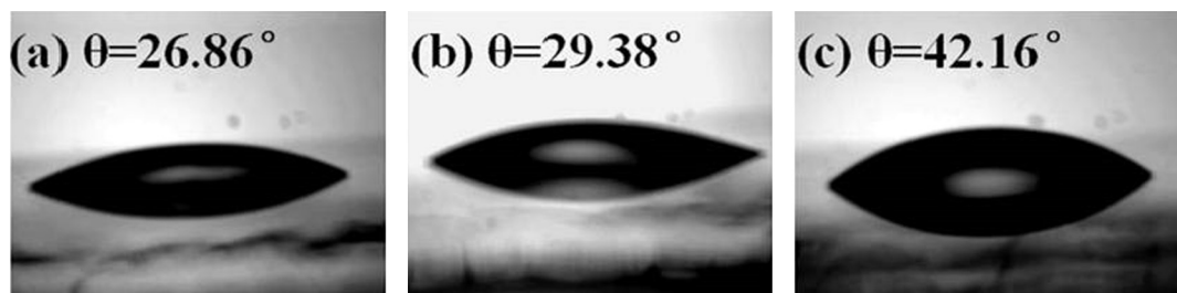
Fig. 3. Contact angles of the water-drops on the surface of (a) bare \text{TiO}_2 , (b) \text{TiO}_2/\text{non-SAM CQD} , and (c) \text{TiO}_2/\text{SAM CQD} films.
