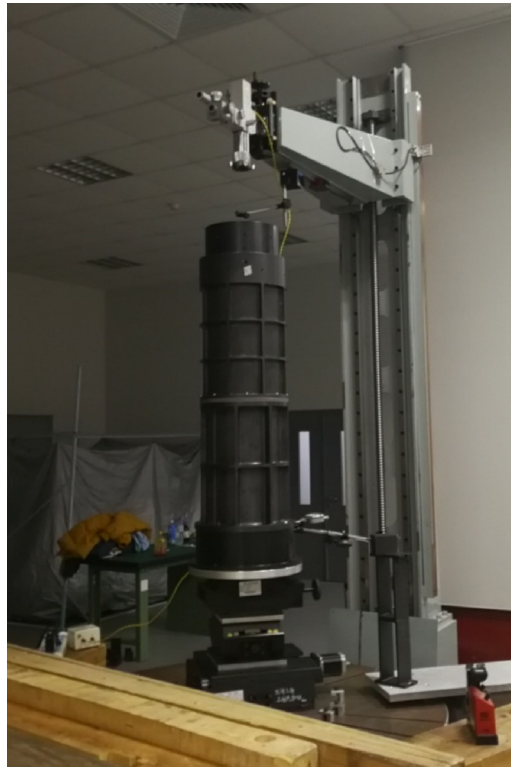
Fig. 15. The lens assembly adjustment on precision lens eccentric instrument.
