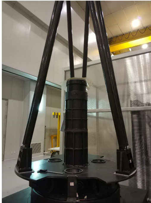
Fig. 16. The lens assembly mounted on the turntable.
