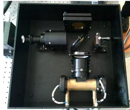
**Fig.11** Simplified configuration of the light FTIRS
