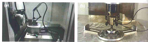
Fig. 1. Direct polishing instruments (a) SPDT, (b) CMP.
