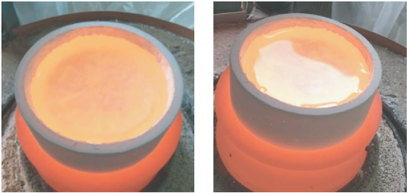
(c)成型及排气泡过程 (c)Forming and exhaust bubble process
