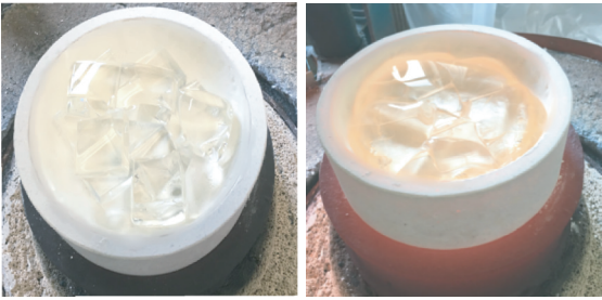
(a)玻璃表层塌陷 (a)Surface of glass was collapsed
