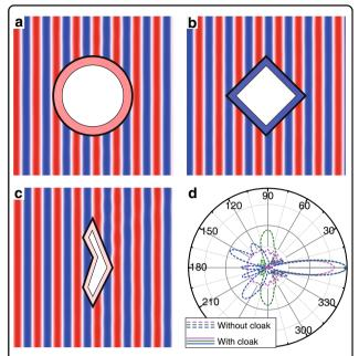
Fig. 2 Numerical demonstrations via the effective medium model. a–c The electric field distributions for the cases of a circular hybrid cloaking shell, a rhombic hybrid cloaking shell, and an irregular hybrid cloaking shell with a complex polygon shape. The illumination source is a TE-polarized plane wave from the left. d The far-field radiation patterns of the scattered waves for the cases in a (purple), b (green), and c (blue) with (solid lines) and without (dashed lines) the cloaking shells
