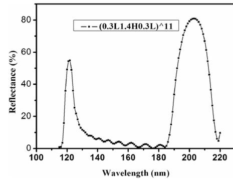
Fig. 3 Theoretical reflectance curve of periodic multilayer (sub/(0.3L1.4H0.3L)<sup>11</sup>/air)
