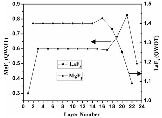
Fig. 6 Thickness distribution of discrete layers of seven layers apodization of multilayer
