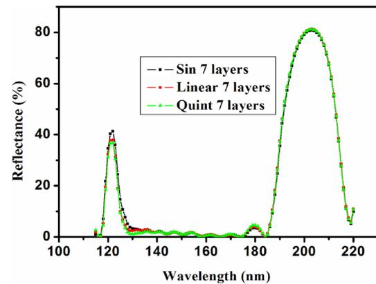
**Fig. 9** Theoretical reflectance curves of three kinds (sine-wave, linear, and quintic functions) of AM-TMD (seven layers apodization)
