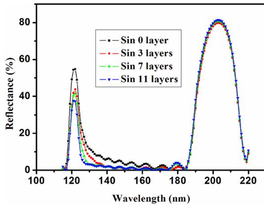
Fig. 5 Theoretical reflectance curves of right side sine-wave AM-TMD of multilayer (zero, three, seven, and eleven layers apodization)
