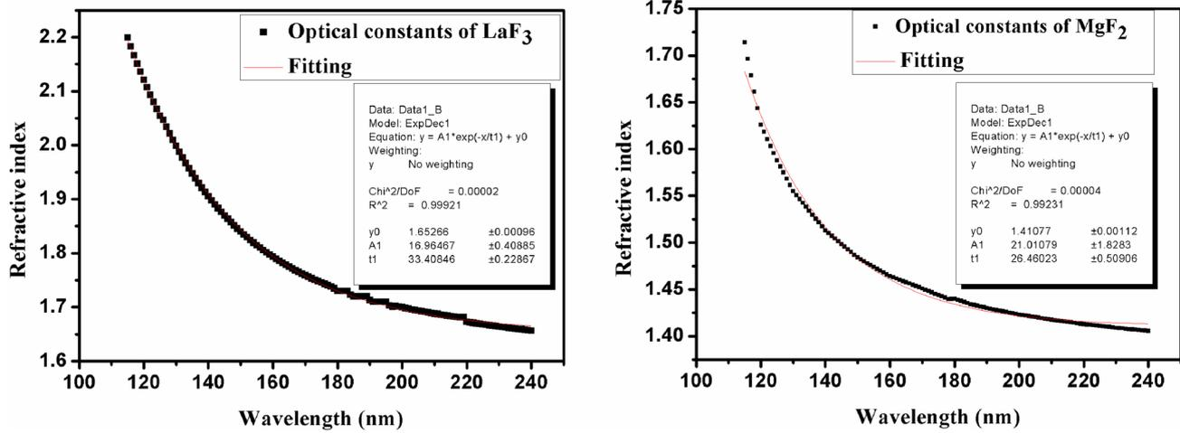
Fig. 2 Fittings of optical constants for LaF<sub>3</sub> (left) and MgF<sub>2</sub> (right) by first-order exponential decay
