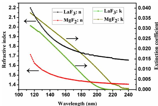
Fig. 1 Optical constants of LaF<sub>3</sub> and MgF<sub>2</sub>
