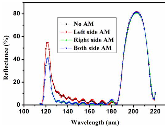
Fig. 4 Theoretical reflectance curves of left side, right side, and both side AM-TMD of multilayer (seven layers apodization)
