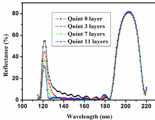
**Fig. 8** Theoretical reflectance curves of right side quintic AM-TMD of multilayer (zero, three, seven, and eleven layers apodization)
