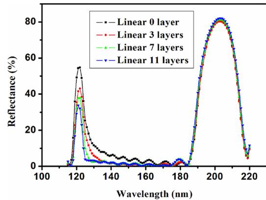
Fig. 7 Theoretical reflectance curves of right side linear AM-TMD of multilayer (zero, three, seven, and eleven layers apodization)
