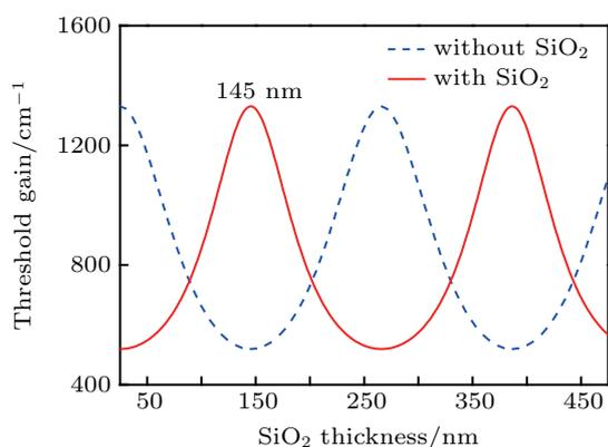
Fig. 1. (color online) Calculated VCSEL threshold gain with (red line) and without (blue line)  $\text{SiO}_2$  layer.
