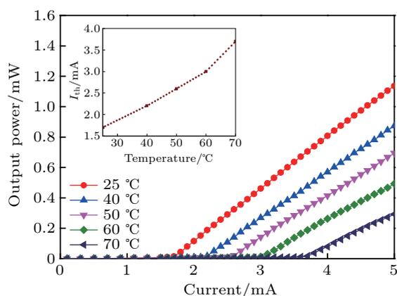
**Fig. 4.** (color online)  $L$ - $I$ - $V$  characteristics and the variation of threshold current (the inset) of the continuous-wave current injection for the VCSEL with a dielectric mode filter.
