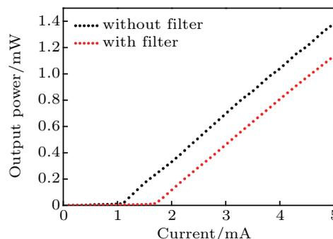
**Fig. 5.** (color online) Comparison of VCSEL output power with and without mode filter.
