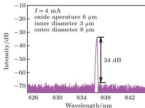
**Fig. 6.** (color online) Spectra of the VCSEL with a dielectric mode filter. The fabricated device is tested under  $I = 4$  mA.
