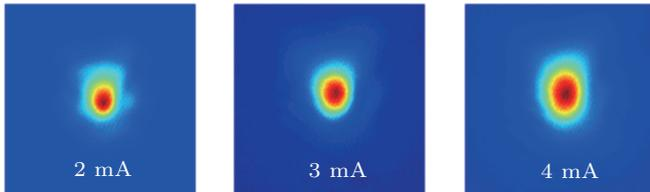
Fig. 7. (color online) Measured near field patterns under different continuous-wave currents  $I = 2, 3,$  and  $4$  mA.
