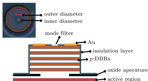
Fig. 3. (color online) Cross section of the VCSEL with dielectric mode filter. The inset is the top view image of the VCSEL with dielectric mode filter. The inner diameter is 3  $\mu\text{m}$  and the outer diameter is 8  $\mu\text{m}$ .
