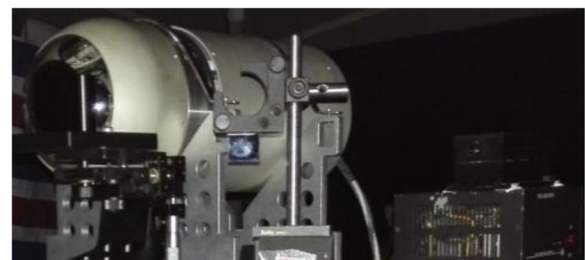
Fig. 16 Seeker optical imaging system simulator
