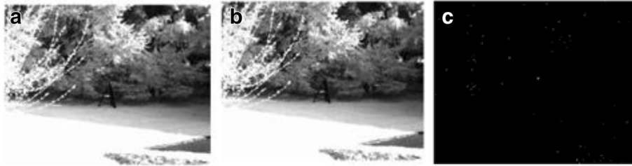
Fig. 14 Image differential processing example. a Passive imaging. b Active imaging. c Differential image
