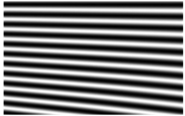
Fig. 6. Results of simulation of the interference fringe caused by the cosine error before cosine error correction.
