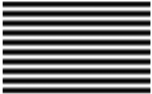
Fig. 8. Results of simulation of the interference fringe caused by the cosine error after cosine error correction.
