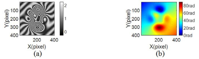
Fig. 5. Simulated interferogram with the complex fringes and reference phase distribution. (a) One of the simulated interferograms, (b) reference phase distribution (PV = 89.375 rad, RMS = 18.359 rad).
