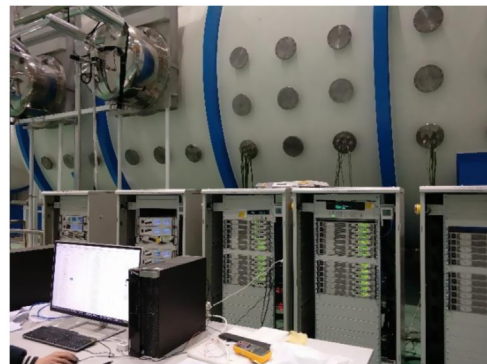
Fig. 14 MTF measurement of the space telescope site.
