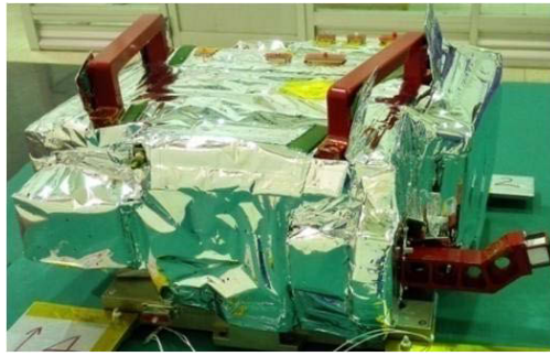
Fig. 18. The photo of the limb hyperspectral imager
