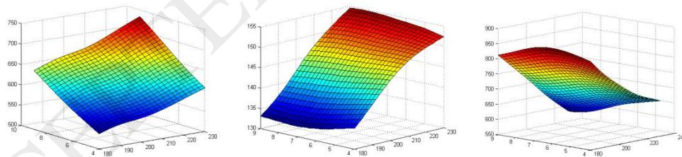
Figure 5 Mapping relation between outputs  $M, f_1, RMS$  and inputs  $x_1, x_2$  ( $x_3=x_4=6\text{mm}$ )
