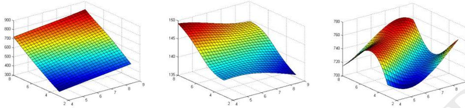
Figure 6 Mapping relation between outputs  $M$ ,  $f_1$ ,  $RMS$  and inputs  $x_2, x_3$  ( $x_1=200\text{mm}$ ,  $x_4=6\text{mm}$ )
