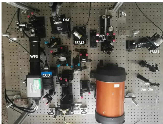
Fig. 10 Optical layout of FSOC with disturbance FSM.
