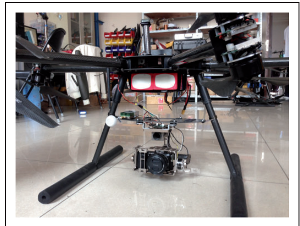
Figure 4. The stable tracking control system of an AOEP mounted on a Hex-Rotor UAV for experimentation.
