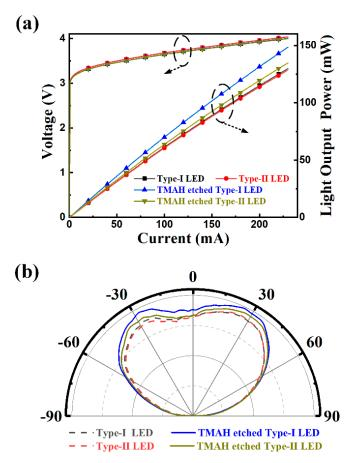
**Figure 6.** (a) *L-I-V* characteristics of the cuboid geometry LEDs with and without TMAH etching treatment. (b) Far-field emission patterns of the cuboid geometry LEDs with and without TMAH etching treatment.
