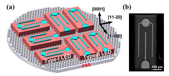
**Figure 1.** (a) Schematic diagram of Type-I LED and Type-II LED with different sidewall orientations. (b) SEM image of the fabricated LED chip.
