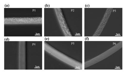
Figure 5. (a–f) SEM images of selected areas of Type-II LED chips, (a) P1; (b) P2; (c) P3; (d) P4; (e) P5; and (f) P6. The six regions were chosen at the same position as they were in the Type-I LED chips.
