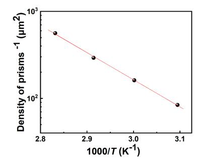
**Figure 3.** The inverse density of prisms plotted as a function of the reciprocal of temperature following the Arrhenius plot fit.
