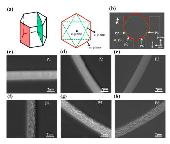
**Figure 4.** (a) Schematic of the wurtzite structure GaN unit cell and its projection in the *c*-plane. (b) SEM images of Type-I LED chips, the projection was incorporated to show the exposed *m*-plane and *a*-plane. (c-h) The SEM images at marked positions: (c) P1; (d) P2; (e) P3; (f) P4; (g) P5; and (h) P6.
