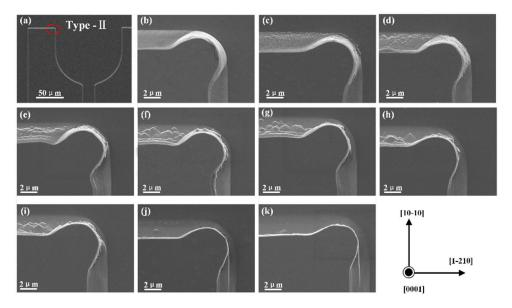
**Figure 2.** (a) SEM images of Type-II LED chips, the marked corner was chosen to show the morphology change after TMAH etching. (b–k) SEM images of the marked corner with different etching time: (b) 0 min; (c) 1 min; (d) 2.5 min; (e) 5 min; (f) 7.5 min; (g) 10 min; (h) 15 min; (i) 20 min; (j) 30 min; and (k) 40 min.
