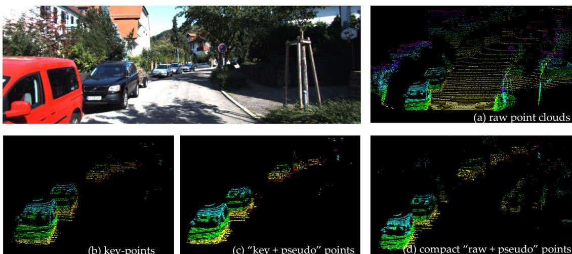
**Figure 9.** Visualizations of the results of key-point densification. (a) is a representative view of raw point clouds. (b) is the view of key-points selected according to our distance preference strategy. (c) is the view of “key + pseudo” points (pseudo-points are generated by K-means from the corresponding image). (d) is the view of compact “raw + pseudo” points reorganized according to our sorting simplification strategy.
