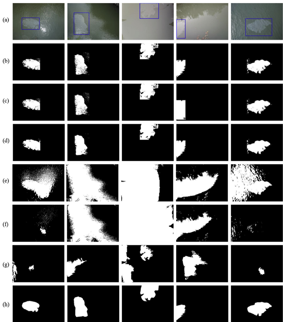
Fig. 5. Segmentation examples of RGB images. (a) Original images (the blue box is a location bounding box), (b) Faster R-CNN + Otsu, (c) Faster R-CNN + Max entropy, (d) Faster R-CNN + LFTM with N_{cluster}=2 , (e) Otsu, (f) Max entropy, (g) improved LFTM (h) ground-truth. (For interpretation of the references to colour in this figure legend, the reader is referred to the Web version of this article.)
