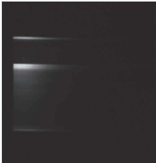
Fig. 11. Fluorescence line image of turbine oil.
