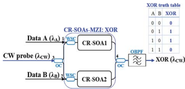
Figure 2. Schematic diagram and truth table of XOR logic gate using CR-SOAs-MZI. OC: 3 dB optical coupler. WSC: wavelength-selective coupler. OBPF: optical bandpass filter.
