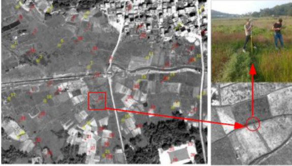
Fig. 11. Measure the control points and check points using RTK method.
