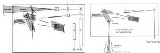
(a) Interferometric system (b) Holographic reconstruction system
