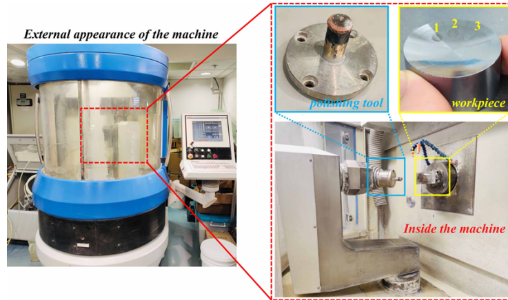
Fig. 10. Spot polishing experiment conducted on Zeeko IRP200 machine.
