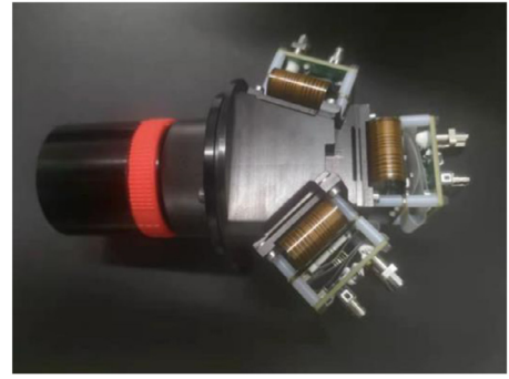
Fig. 5. The optical system prototype. The imaging effect in the water was carried out by standard color, which is put in the water under the distance of 0.5 m. The final image is demonstrated in Fig. 8 which shows very high color reducibility.
