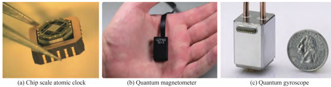
图4 量子精密测量装置实物 [35,42-43] Fig.4 The Quantum precision measurement devices [35,42-43]
