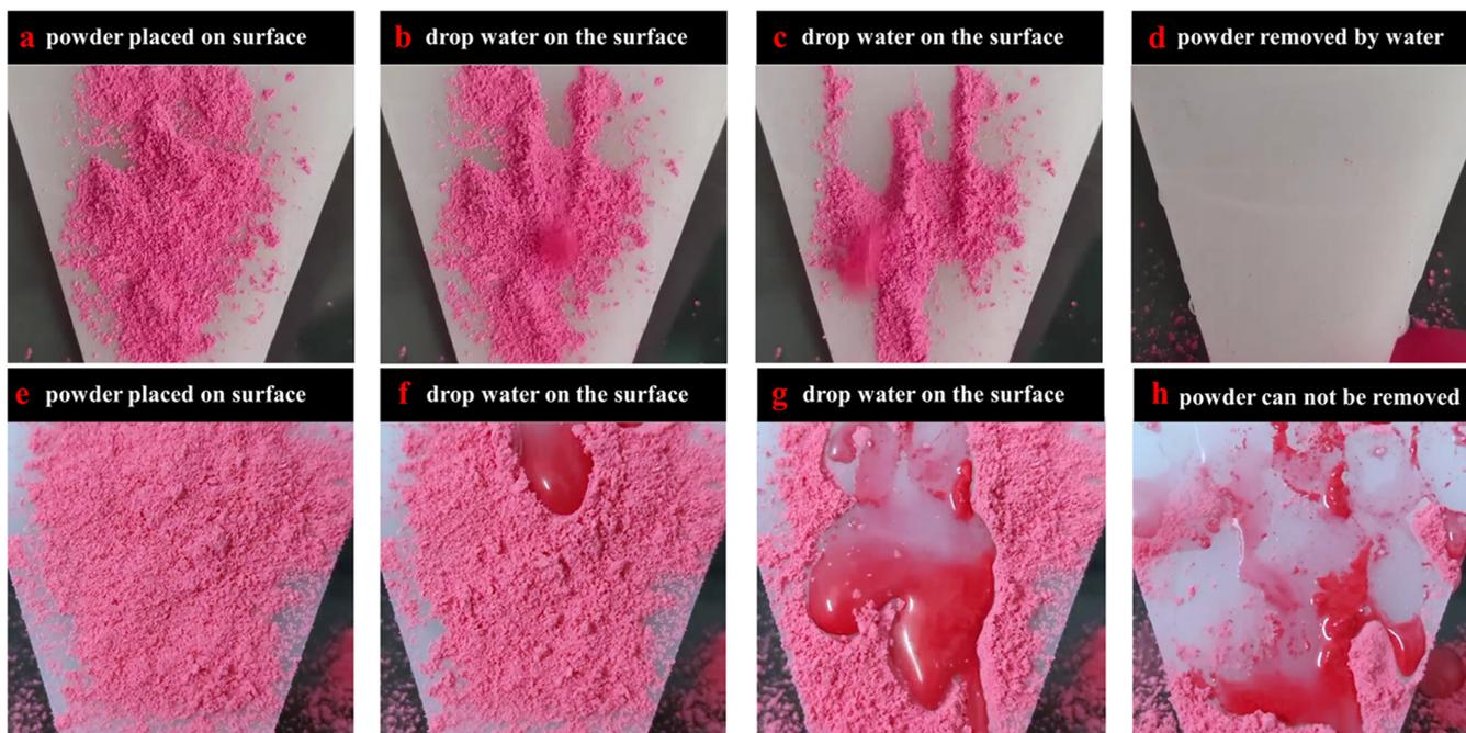
**Figure 7.** Self-cleaning test with powder on the imprinted (a–d) and untreated (e–h) PP surface: (a) powder particles are put on the imprinted surface; (b, c) water is dropped on the imprinted surface; (d) powder particles are removed out of the surface by water droplets; (e) powder particles are put on the untreated surface; (f, g) water is dropped on the untreated surface; and (h) powder particles cannot be removed out of the surface by the water droplets.
