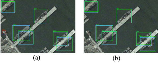
Fig. 18. Ship detection results with OHgN compared to HgN. The blue box denotes the ground truth, the green box denotes TP, the red denotes FP, and the pink denotes FN. With SENet, the false detection of ships can be effectively reduced. (a) HgN+TBHN. (b) OHgN+TBHN. (a) Ship detection results on CS measurements of HgN+TBHN. (b) Ship detection results on CS measurements of OHgN+TBHN.
