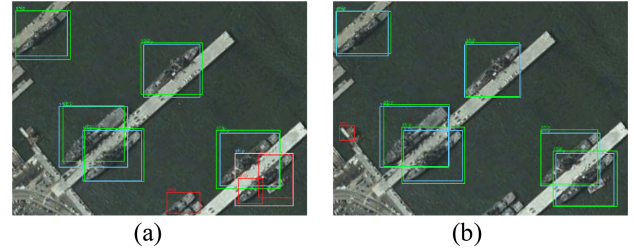
Fig. 17. Ship detection results with HgN compared to ResNet50. The blue box denotes the ground truth, the green box denotes TP, the red denotes FP, and the pink denotes FN. With HgN, the correct ship position can be detected effectively. (a) ResNet50+TBHN. (b) HgN+TBHN. (a) Ship detection results on CS measurements of OHgN+TBHN. (b) Ship detection results on CS measurements of HgN+TBHN.
