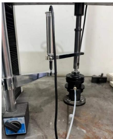
**Figure 8.** HSU on the testing machine.
