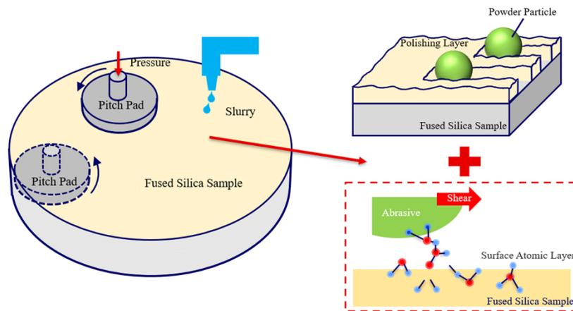
**Fig. 1.** Schematic diagram of CCOS processing.
