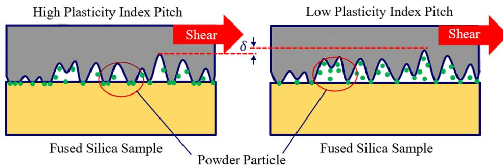
**Fig. 12.** The contact situation of pitch with different plasticity index and fused silica.
