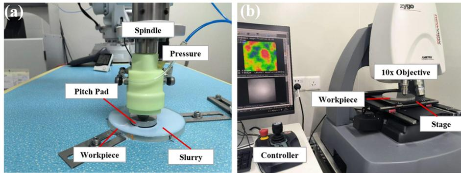
**Fig. 6.** Processing and testing device. (a) CCOS processing process; (b) testing process.
