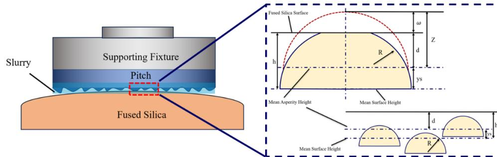
**Fig. 2.** Contact between pitch and fused silica surface.
