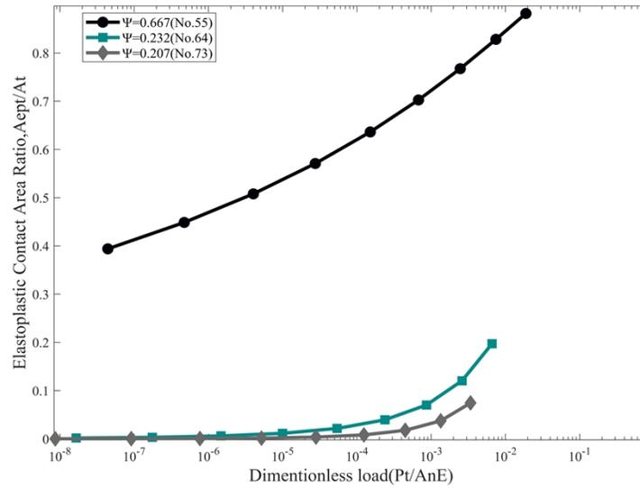
**Fig. 3.** The relationship between elastic-plastic contact and real contact area ratio  $A_{ept}/A_t$ , dimensionless load  $P_t/A_n E$  and plastic exponent  $\psi$ .
