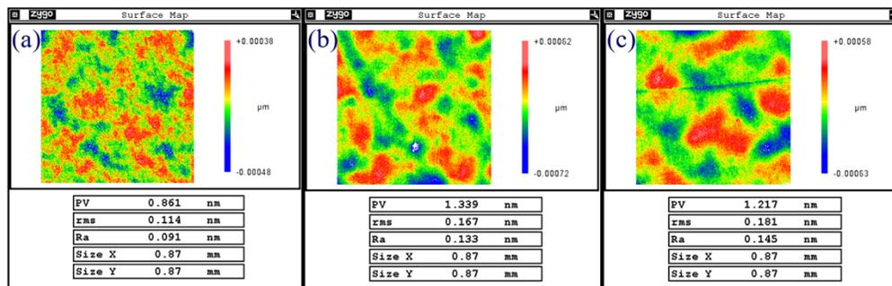
**Fig. 8.** Surface roughness of fused silica polishing for 60 minutes. (a) Surface roughness of No. 55 pitch after polishing; (b) Surface roughness of No. 64 pitch after polishing; (c) Surface roughness of No. 73 pitch after polishing.
