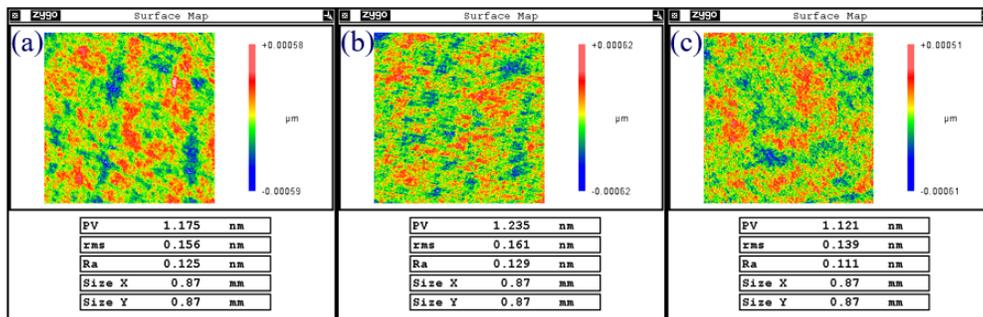
**Fig. 7.** Initial surface roughness of fused silica. (a) Surface roughness of No. 55 pitch before polishing; (b) Surface roughness of No. 64 pitch before polishing; (c) Surface roughness of No. 73 pitch before polishing.
