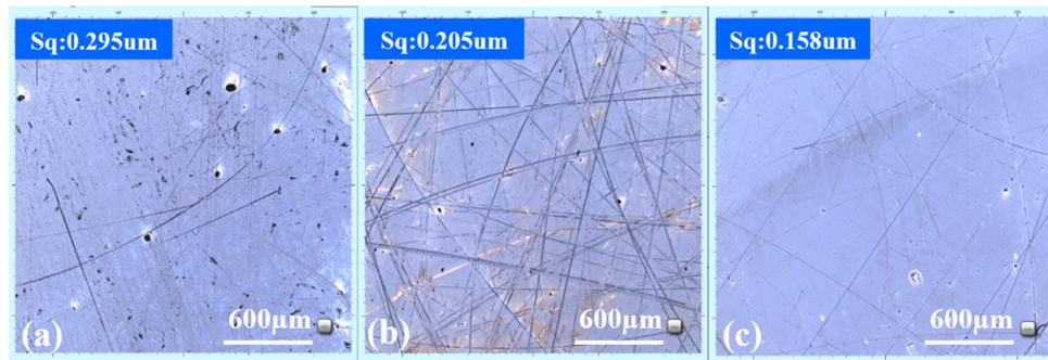
**Fig. 11.** Morphology of three kinds of pitch after processing. (a) Surface morphology of No. 55 pitch; (b) Surface morphology of No. 64 pitch; (c) Surface morphology of No. 73 pitch.
