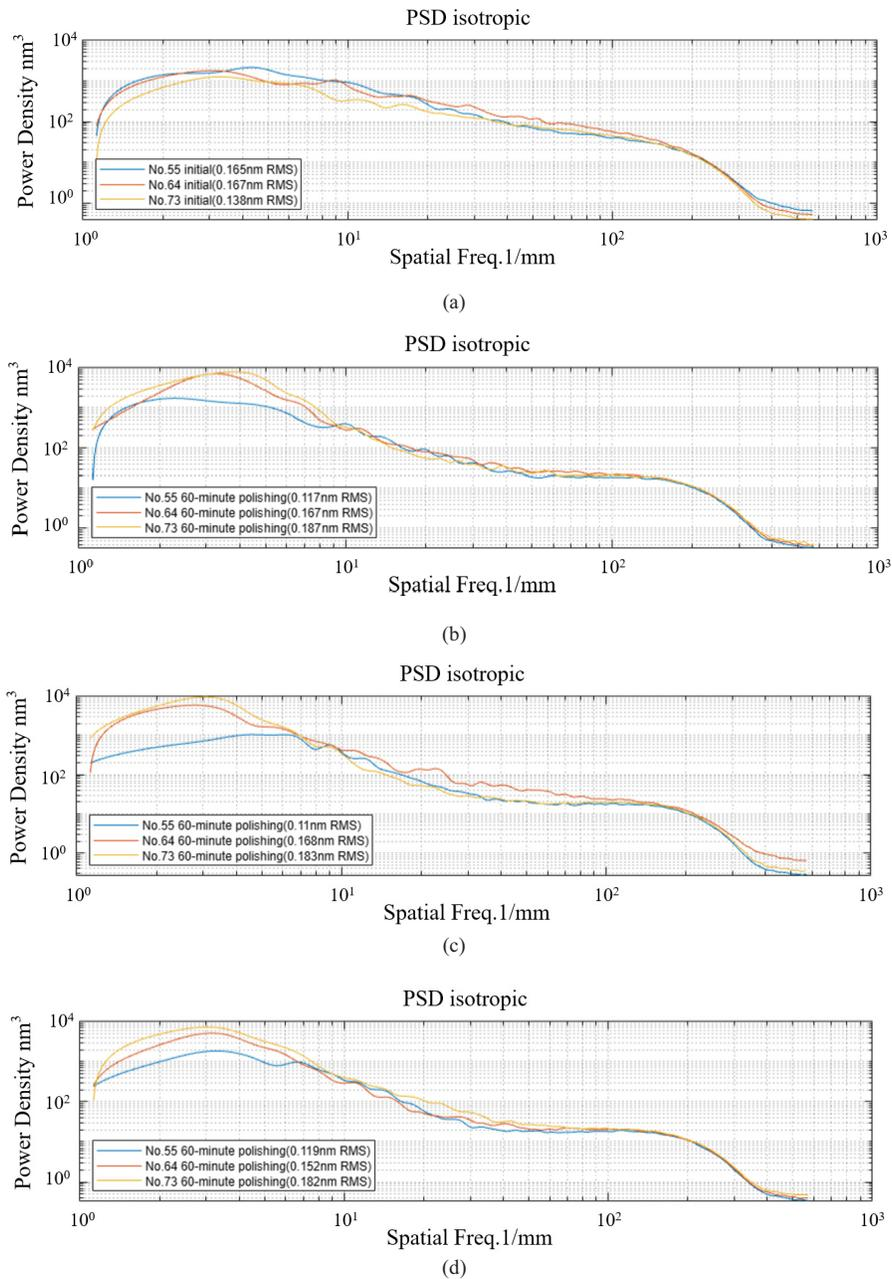
**Fig. 9.** PSD curves of different sampling points of three kinds of pitch. (a) PSD curves at the center of the mirror before polishing with three types of pitch; (b) PSD curves at the center of the mirror after polishing with three types of pitch; (c) PSD curves at a distance of 20 mm from the center of the mirror after polishing with three types of pitch; (d) Three PSD curve at 40 mm from the center of the mirror after polishing with three types of pitch.
