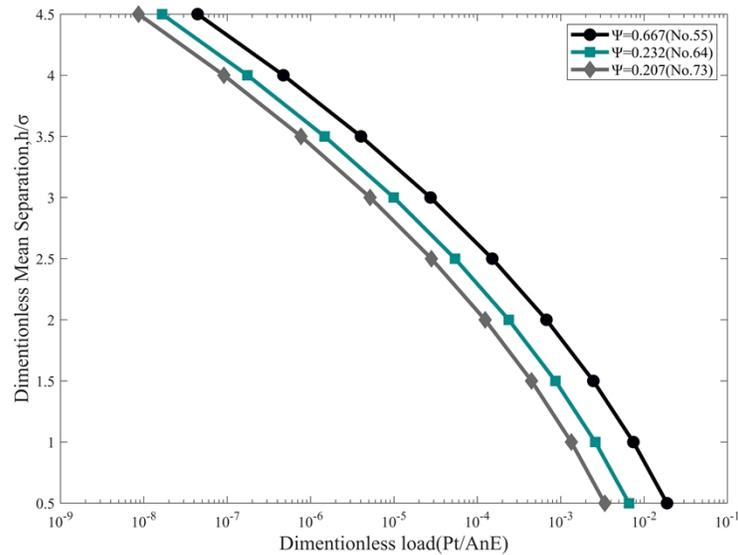
**Fig. 5.** Variation of dimensionless  $h/\sigma$  with  $P_t/A\eta E$  under different plastic exponents  $\psi$ .
