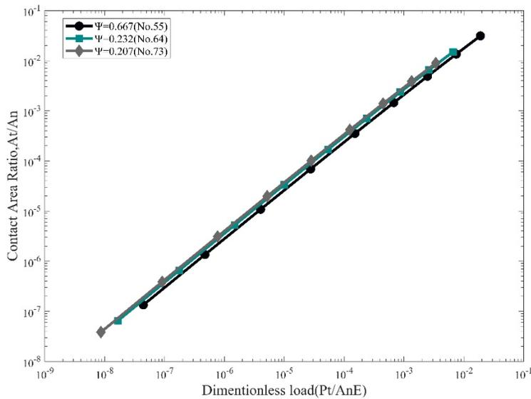
**Fig. 4.** Relationship between real contact area ratio  $A_t/A_n$ , dimensionless load  $P_t/A_n E$  and plastic exponent  $\psi$ .
