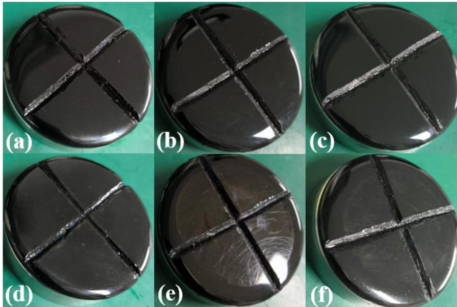
**Fig. 10.** Changes of surface morphology of three kinds of pitch before and after processing. (a) Before polishing No. 55 pitch; (b) After polishing No. 55 pitch; (c) Before polishing No. 64 pitch; (d) After polishing No. 64 pitch; (e) Before polishing No. 73 pitch; (f) No. 73 pitch After pitch polishing.
