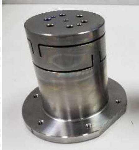
Figure 4. Machined test piece of the flexural mount.
