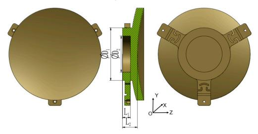
Figure 3. Fundamental structure of the mirror.
