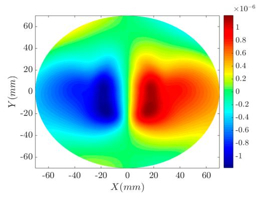
**Figure 5.** Surface shape error in X direction.
