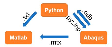
Figure 2. Data interaction diagram.
