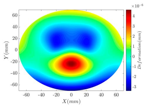
**Figure 7.** Surface shape error in Z direction.
