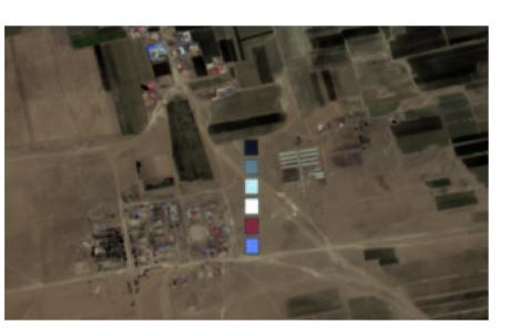
Figure 4. The spatial layout of the radiometric calibration tarps in this study at Baotou site.
