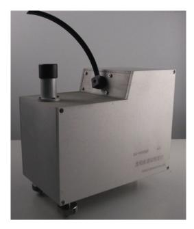
Figure 6. AG-512 SSIR Solar Spectroradiometer.
