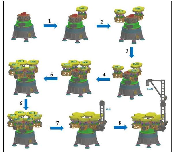
**Figure 10.** Assembly process of the space telescope.
