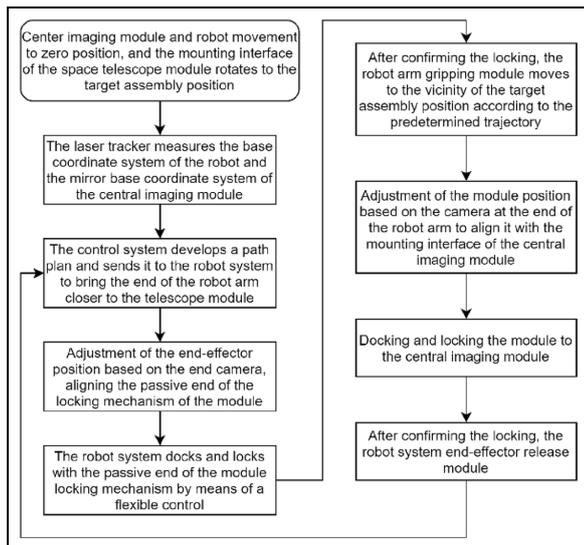
**Figure 11.** Flowchart of the operation of the modules of the robotic manipulator assembly.
