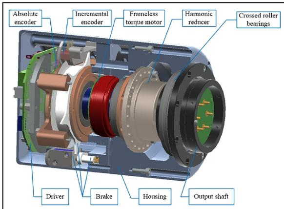
**Figure 4.** Schematic diagram of the internal structure of the joint.
