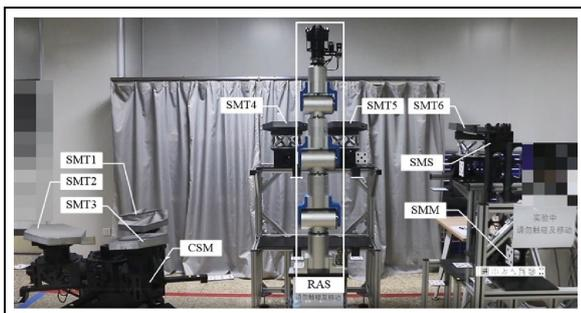
**Figure 12.** Experimental setup for the assembly of a space telescope.
