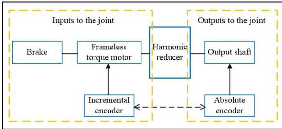
**Figure 3.** Schematic diagram of joint function.
