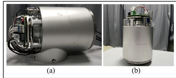
**Figure 5.** Physical view of the joints: (a) horizontal joint and (b) vertical joint.
