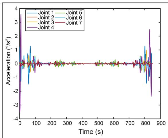
**Figure 17.** Variation of joint angular accelerations with time during the assembly of SMT4 by the redundant robotic manipulator.
