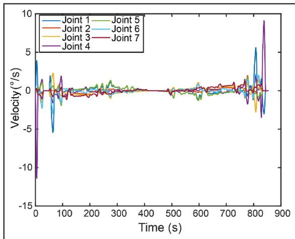
**Figure 16.** Variation of the joint angular velocities of the redundant robotic manipulator with time during the assembly of SMT 4.
