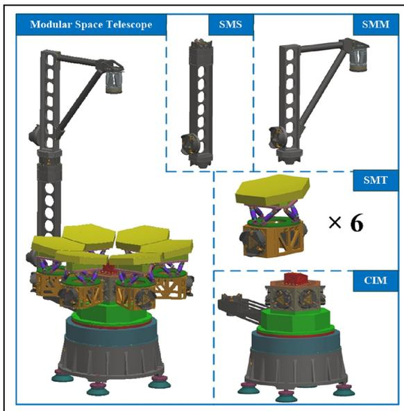
Figure 8. Modular space telescope system.
