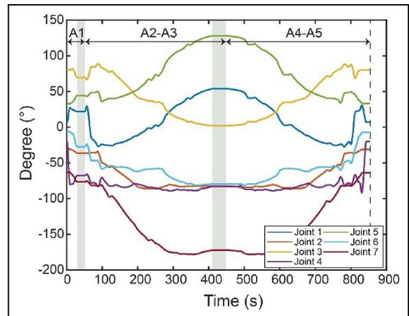
**Figure 15.** Variation of the joint angles of the redundant robotic manipulator during the assembly of SMT4 with time, where the gray area indicates the locking and releasing process of the module.
