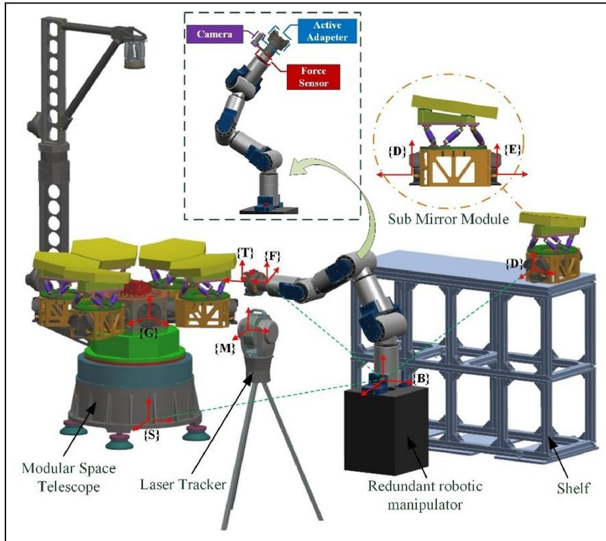
**Figure 9.** System and established coordinate system for ground-based on-orbit assembly demonstration of space telescopes based on robotic manipulators.
