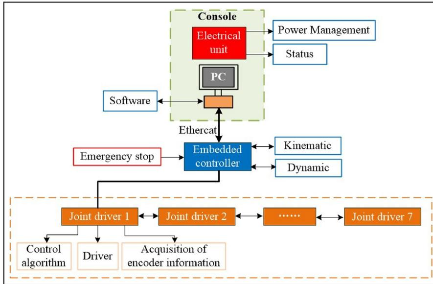
Figure 6. Block diagram of the electrical system of the robotic manipulator.
