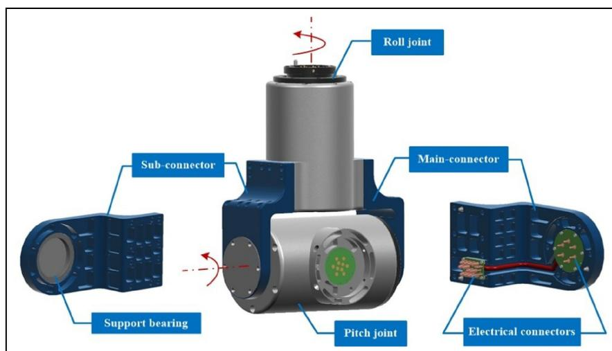
**Figure 2.** Diagram of joint assembly.
