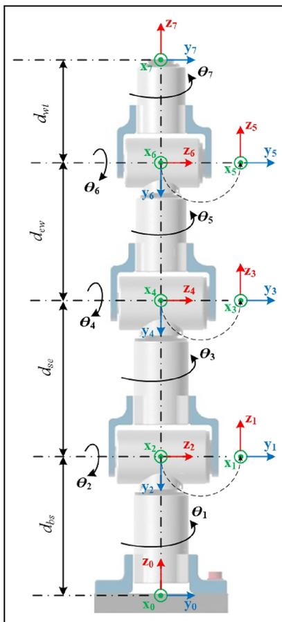
Figure 7. Definition of the robotic manipulator coordinate system.
