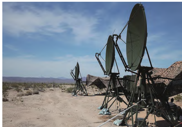
Fig.5 AN/TRC-170 tropospheric scatter microwave radio terminal 图5 AN/TRC-170对流层散射微波无线电终端
