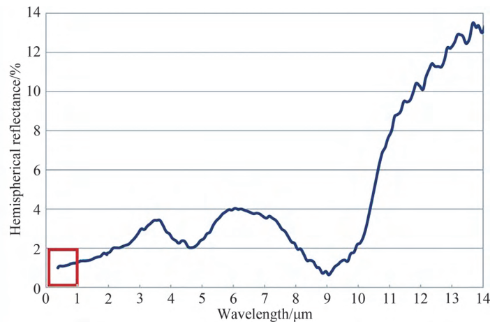
图 16 吸光膜反射率与波长关系 Fig.16 Relation between reflectance of absorbent film and wavelength
